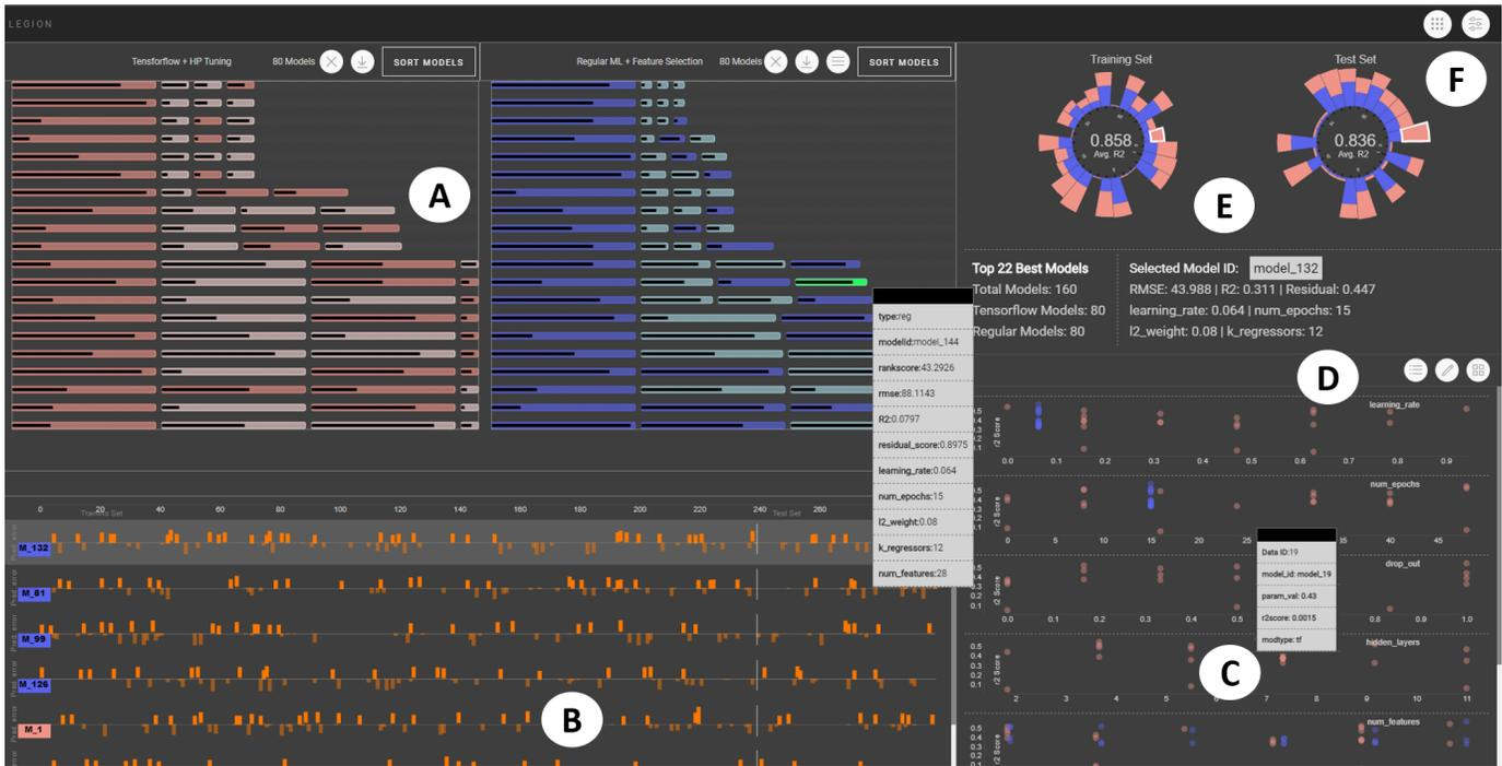
Fig. 1. LEGION - multi-regression modeller. A. Stacked Horizontal Bar View showing regression models constructed using two techniques in separate bins (blue and red bars). B. Instance Unit View. C. Parameter Comparison View. D. Model description in text. E. Radial View showing top 'k' models' RMSE on train and test set (color coded by modeling strategy used). F. Buttons to toggle new models and control panel.
